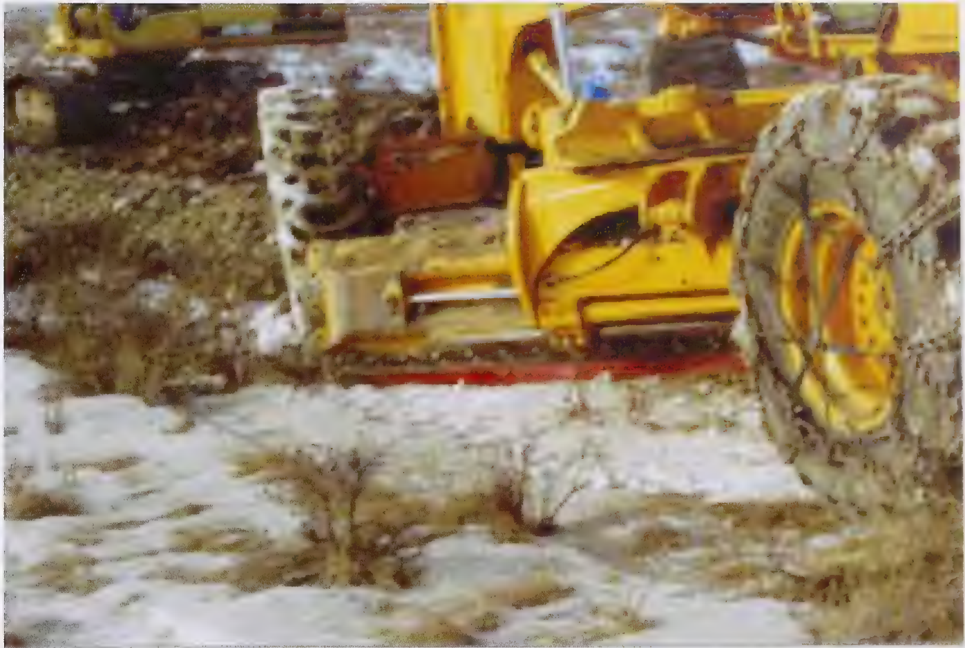
Photo 52 Prairie Protector Blade mounted on a grader blade.
